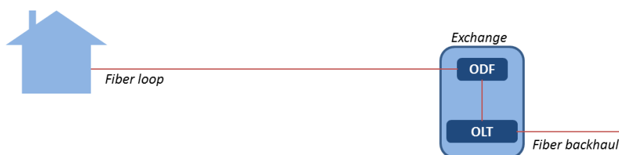
Figuur - Fiber to the Home - scenario Point-to-Point
